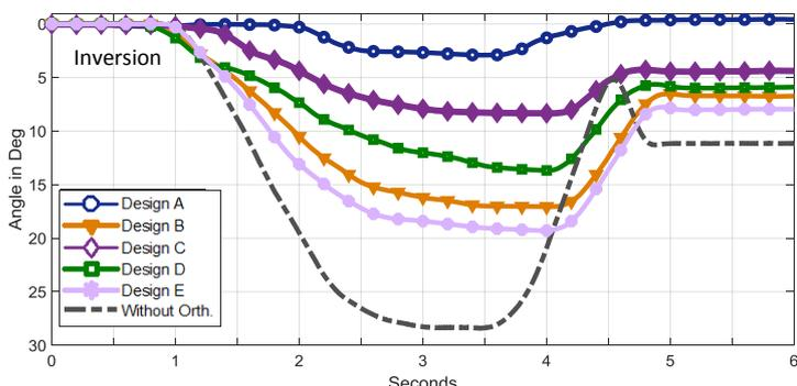
**Fig. 2: Results of dynamic inversion ankle brace test (mean graphs, n=3)**
