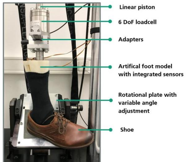
Fig. 1: Machine setup with artificial foot model
