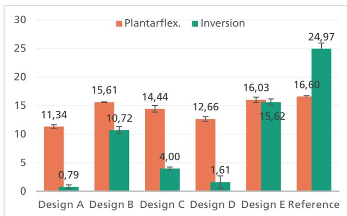
**Tab. 2: Max. inversion & plantarflexion angle (°) - mean (n=3 trials)**
